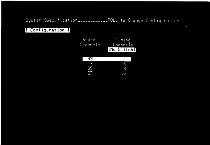
Figure 3-18. State Analyzer System Configuration
